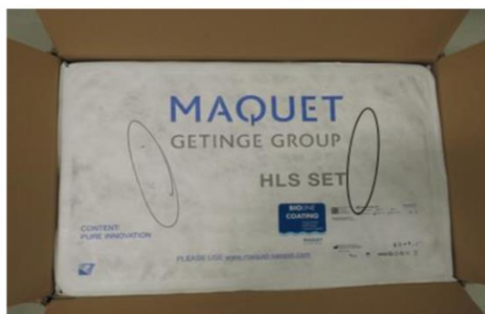
Figure 3: position of potential damages either on left or right side, depending on position of HLS Module in the package
